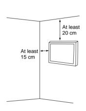
■ Do not block the ventilation holes, and be sure to leave sufficient space around the unit for ventilation.
